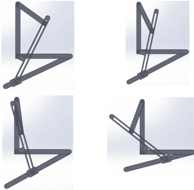
Fig. 6.98 Animation of the four positions of the mechanism
