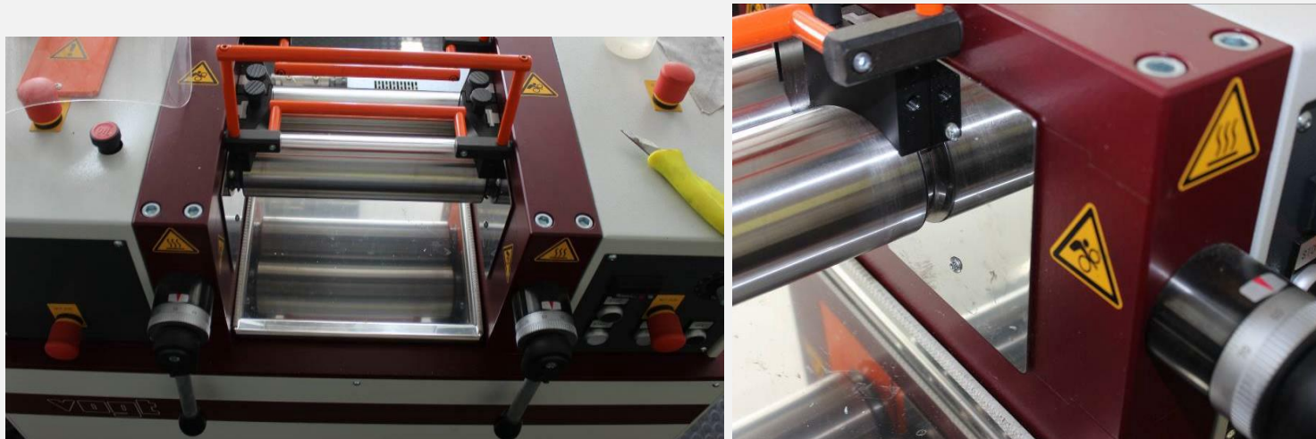
Figure 4. Homogenization machine with detail of rotating heated rollers and hot parts (right)
