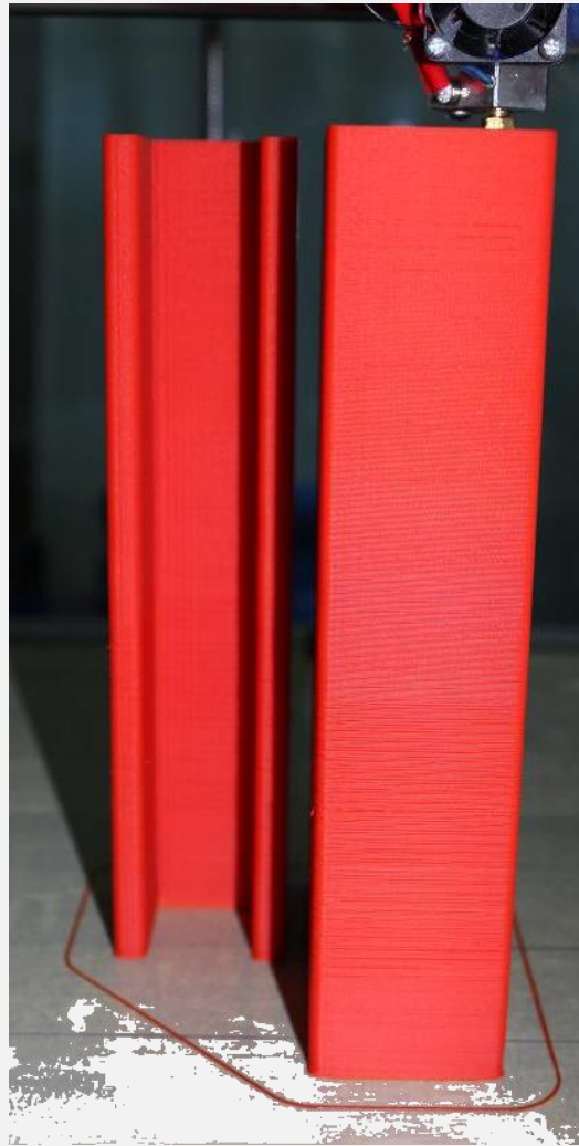
Figure 16. Profiles from PLA – printing of both parts altogether and sequentially
