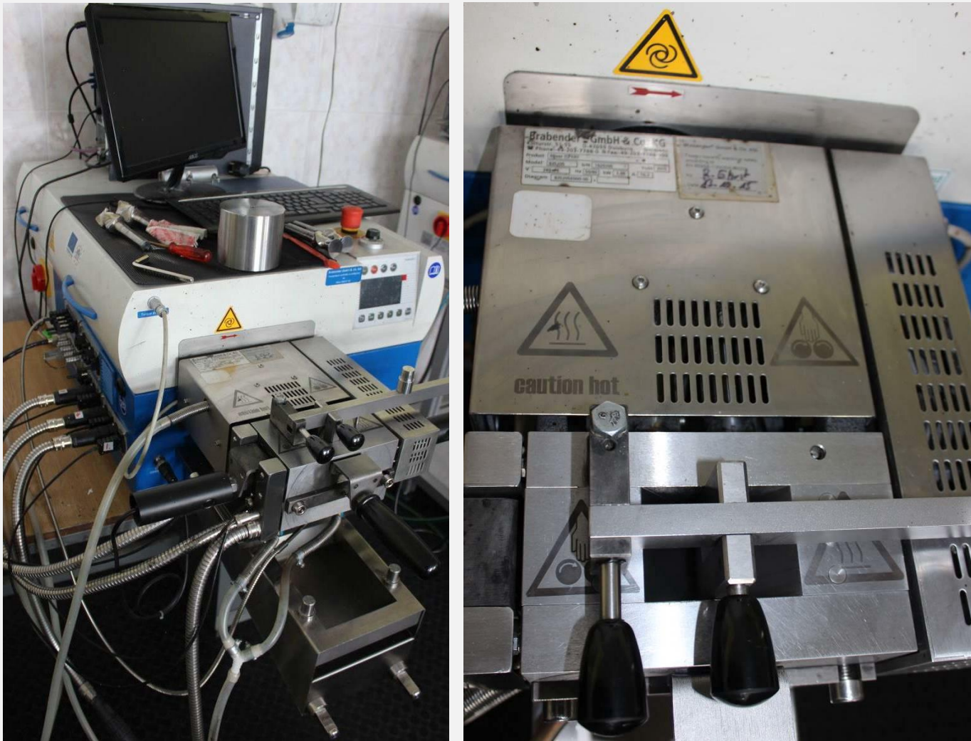
Figure 3. Torque rheometer with detail of hot chamber with pictograms
