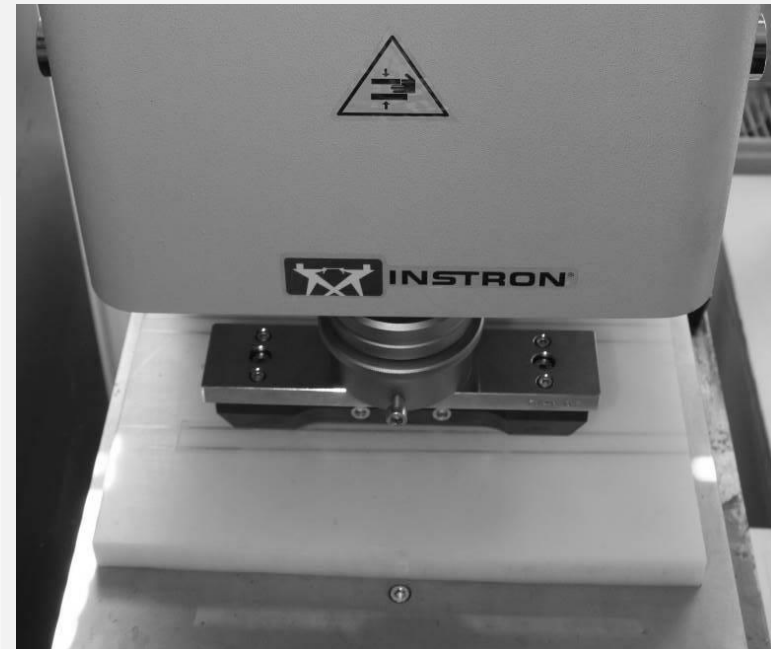
Figure 6. Pneumatic device for the production of test samples with shape of samples (left)
