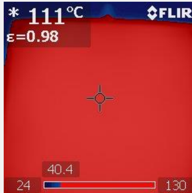
Figure 9. Heated bed temperature – comparison between temperatures set to 120 °C at display and real state on heated bed (thermogram on the right)
