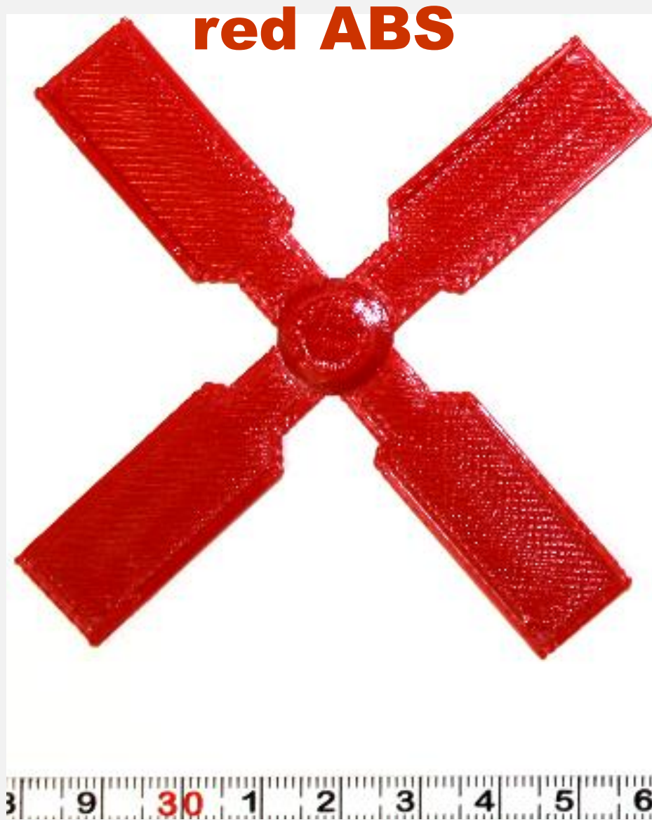
Propeller of model of watermill from red ABS (with tape measure in cm) with its use for kid stuff money-box
