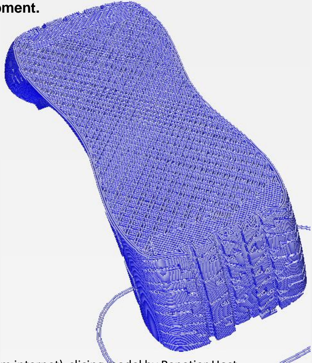
Tire model – design 3D geometry model (from internet), slicing model by Repetier Host
