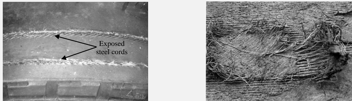
Figure 14. Extreme wear of tire on tread surface; and “cords working-up” (right-photo by Prof. Janíček, VÚT Brno, Czech Republic)
