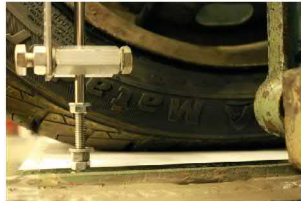
125 % of LI Deformation is 27.5 mm
