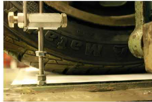
75 % of LI Deformation is 16.4 mm
