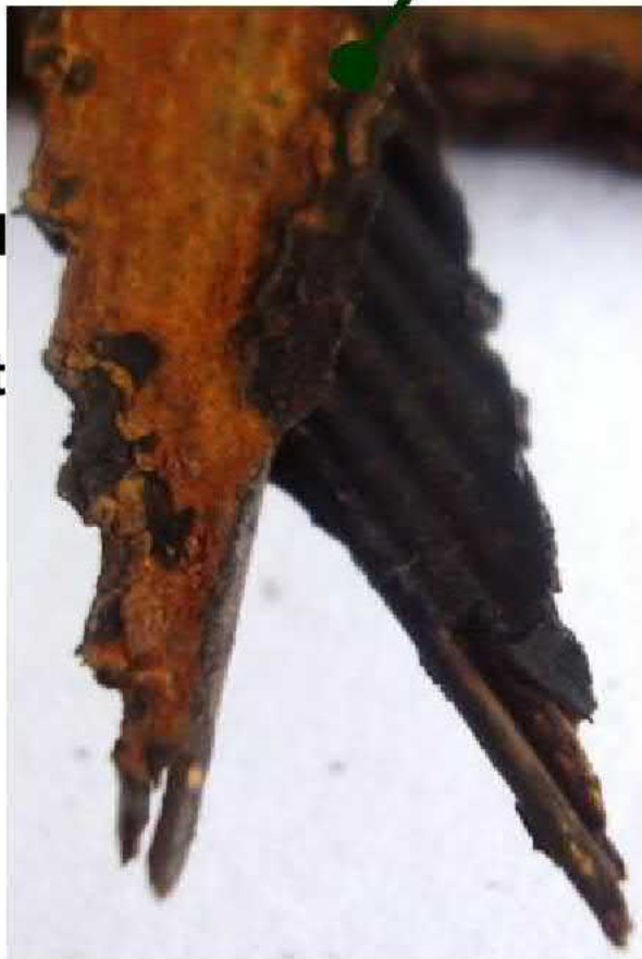
Fig.1. Specimens of steel-cord belt after failure with details of fracture area.
