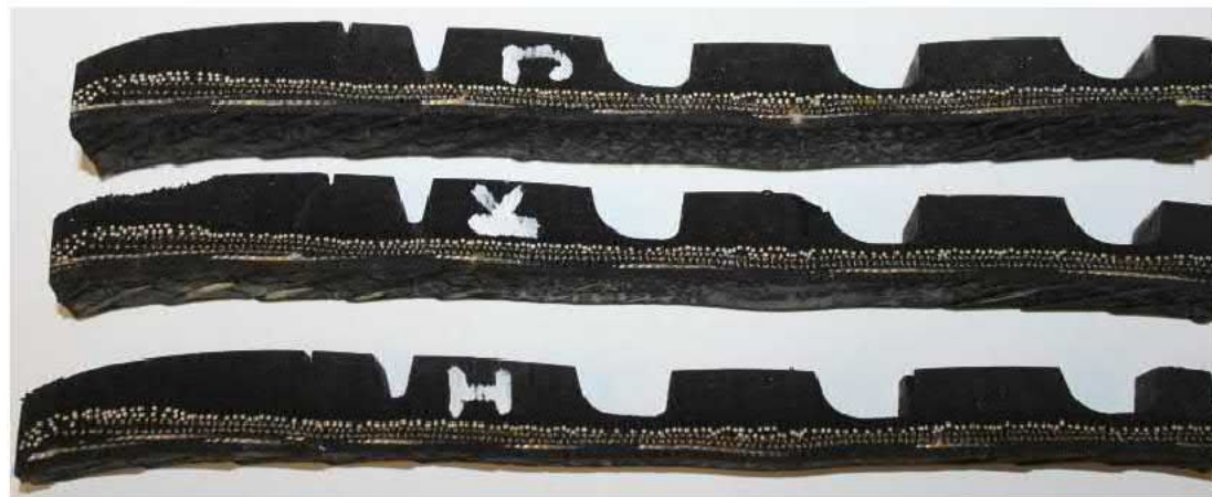
Specimens - cuttings in longitudinal direction (up) and transverse direction (down) with different width, prepared for performance of the tensile and bend tests
