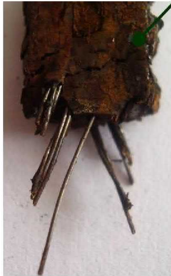
Fig.1. Specimens of steel-cord belt after failure with details of fracture area.
