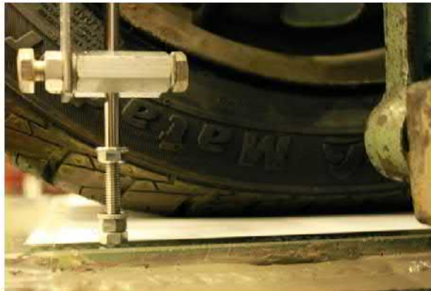
100 % of LI Deformation is 22.5 mm
